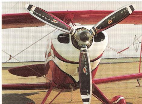
determine the prop's torsional inputs on the crankshaft showed tremendous reductions in stress on the engine during strenuous aerobatic operation. The end result is a subsequent reduction in expensive engine work. With more thrust, better climb, faster acceleration, and reduced torque loads on the engine, the Hartzell system can definitely make a positive impact on your flying.
