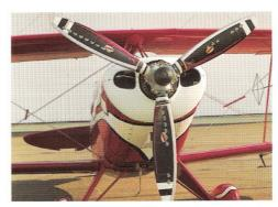
inputs on the crankshaft showed tremendous reductions in stress on the engine during strenuous aerobatic operation. The end result is a subsequent reduction in expensive engine work. With more thrust, better climb, faster acceleration, and reduced torque loads on the engine, the Hartzell system can definitely make a positive impact on your flying.
